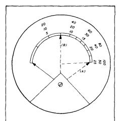
fig. 10. Typical RF power meter scale. For illustrative purposes, point A is the full power (key down) position. Point B is the maximum point at which the indicator should be when operating SSB for the same power output condition.
